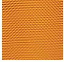
Figure 6. AFM image of mica atoms at 200°C (FFT filtered). 16nm x 16nm.
