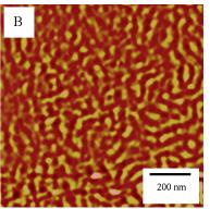
Figure 7. (a) Height and (b) Friction Images of Polystyrenepolybutadiene-polystyrene (PS-PB-PS) block copolymer. z range: 20 nm.
