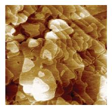
Figure 5. AFM image of Au(111) surface showing monolayer terraces. 2µm x 2µm.
