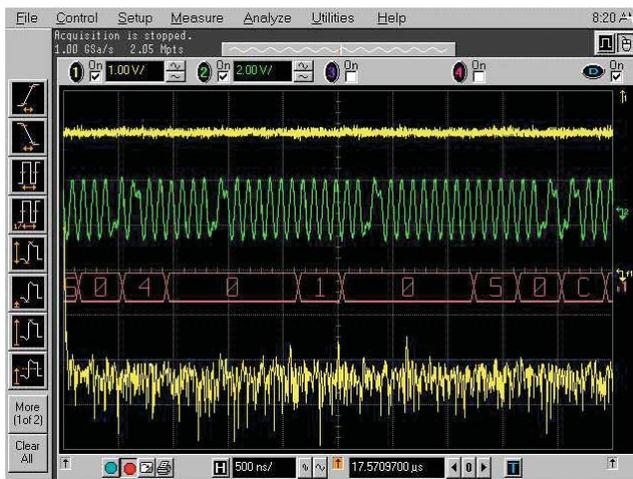
**Figure 14.** Using the MSO's digital channels can help you gain further insight into the possibility of coupling. Moving the horizontal delay back and forth showed that the noise spikes on the FFT changed in magnitude based on which data was present on the LAN signal according to the hex readouts of the digital bus.
