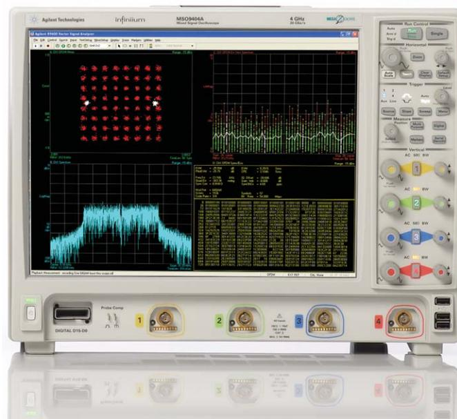
**Figure 13.** Demodulate the WLAN IF signal with the Infiniium 9000 Series oscilloscope.
