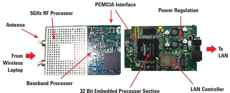
Figure 2. 802.11a 54-Mbps access point with boards unfolded.
