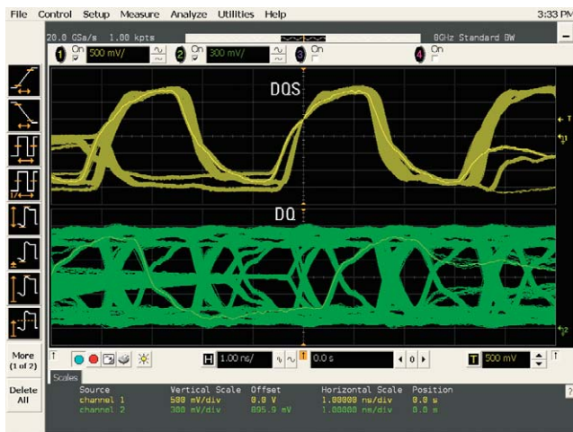
Figure 6. The DDR signal shows a distinctive read and write signal pattern in infinite persistence mode.
