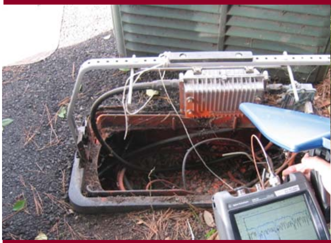
Figure 1a. FieldFox connected to a directional antenna for locating a source of radio interference
