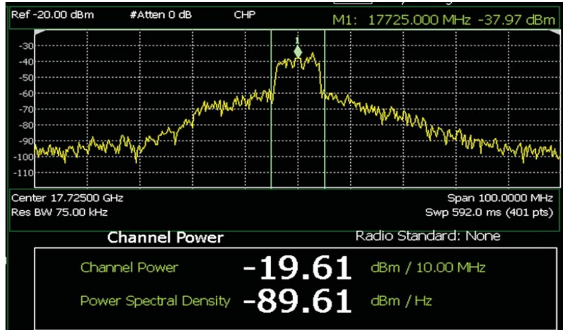
Figure 7a. Channel power measurement
