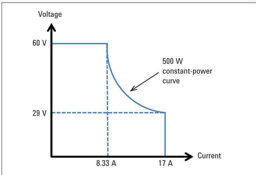
Figure 1. Autoranging output characteristic
