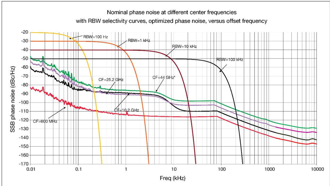
Figure 1. Nominal phase noise at different center frequencies.
