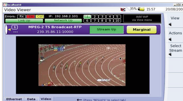
Figure 4: Example of IPTV Video Stream test
