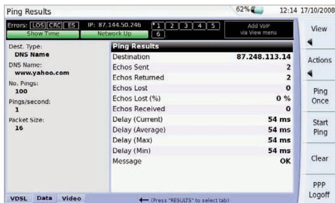
Figure 7: IP Ping test interface
