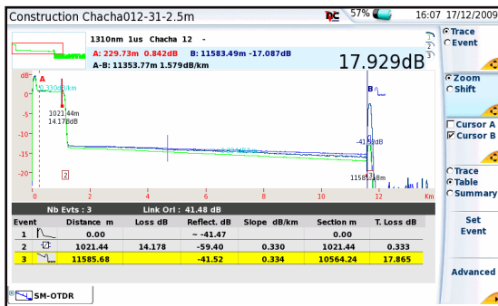
PON system measurement from the customer premises
