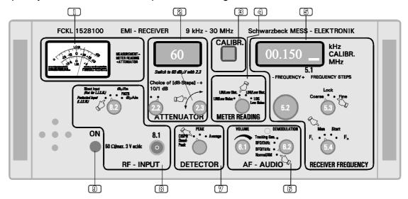
The receiver is now ready to use and frequency is tuned by rotating the encoder (5.2). The steps can be selected with (5.3) fine or coarse.
