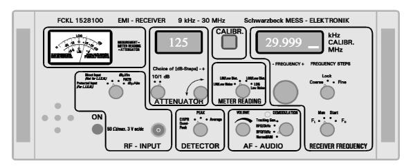
Interference measuring receiver for front panel operation with or without xy-recorder
